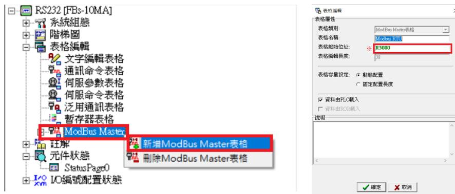
※The form's starting address must be the same with that of the register from the SR command
