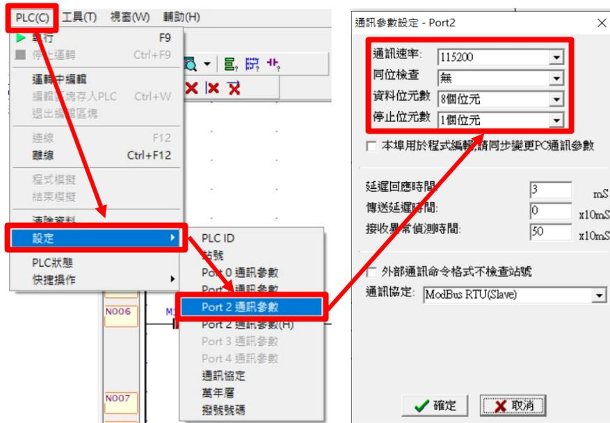
※ This demonstration utilizes communication module CB55 RS485 with Port2 in its address
